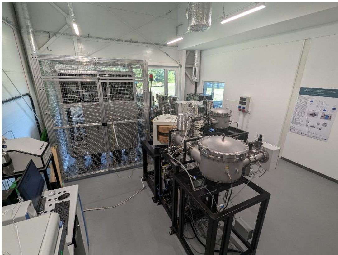
Fig. 2. Positive Ion Mass Spectrometer (PIMS) in the AGH Laboratory for Environmental Radioisotope Analyses (LERA) in Miękinia. Photo: J. Pawlyta
